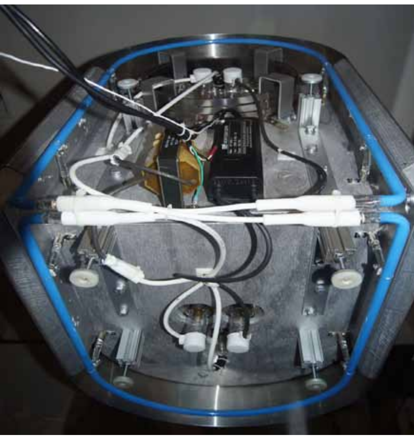
Underside of Illuminated Fountain showing mounting structure and backlighting tubes.
